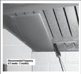
Figure 39 - Clean Behind Tube Scraper
